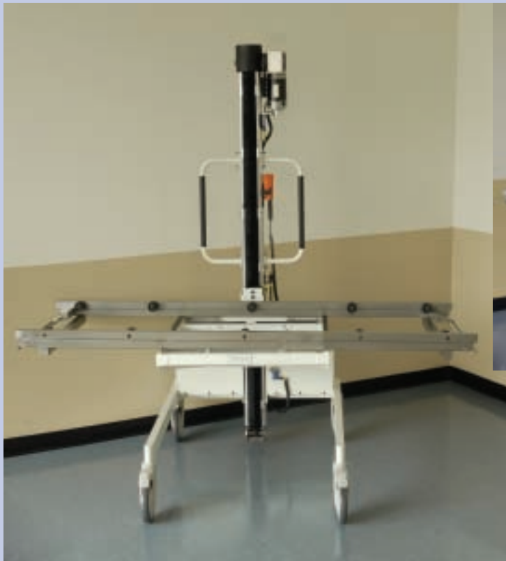
JD1000 shown with JC100 Body Tray and JD400 Roller Pallet. Activation button on flexible cord allows lifting from various positions
